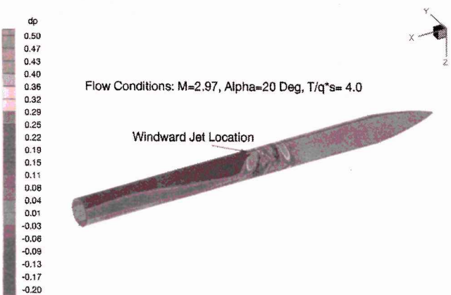
Fig. 12 Surface pressure differential for normal windward jet and jet-off conditions.
