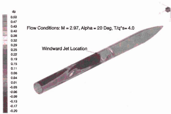
Fig. 16 Surface pressure differential for 30-deg windward forward jet and jet-off conditions.
