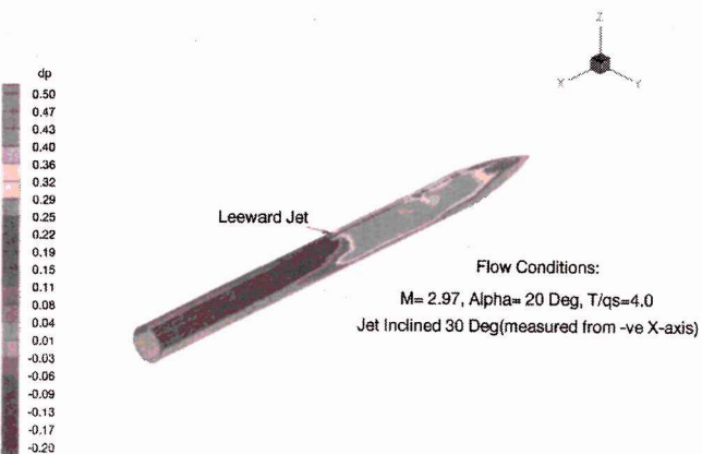
Fig. 15 Surface pressure differential for 30-deg forward leeward jet and jet-off conditions.
