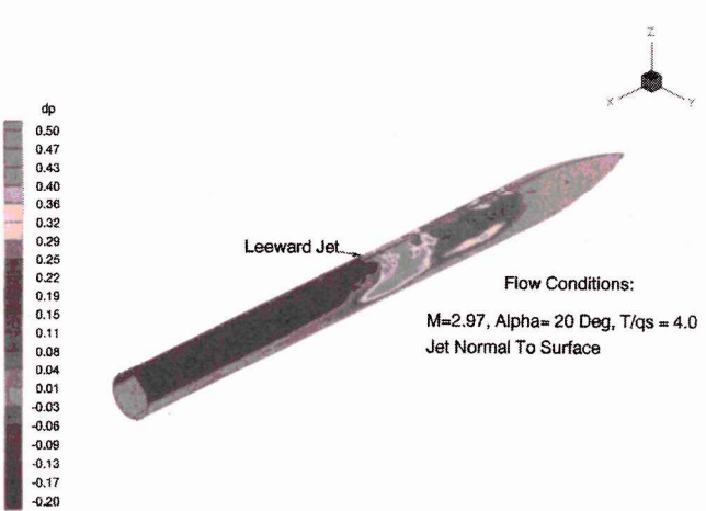
Fig. 14 Surface pressure differential for normal leeward jet and jet-off conditions.
